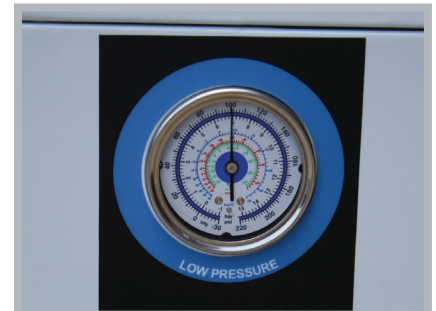
standard refrigerant gauge located on side of cabinet for ease of troubleshooting
